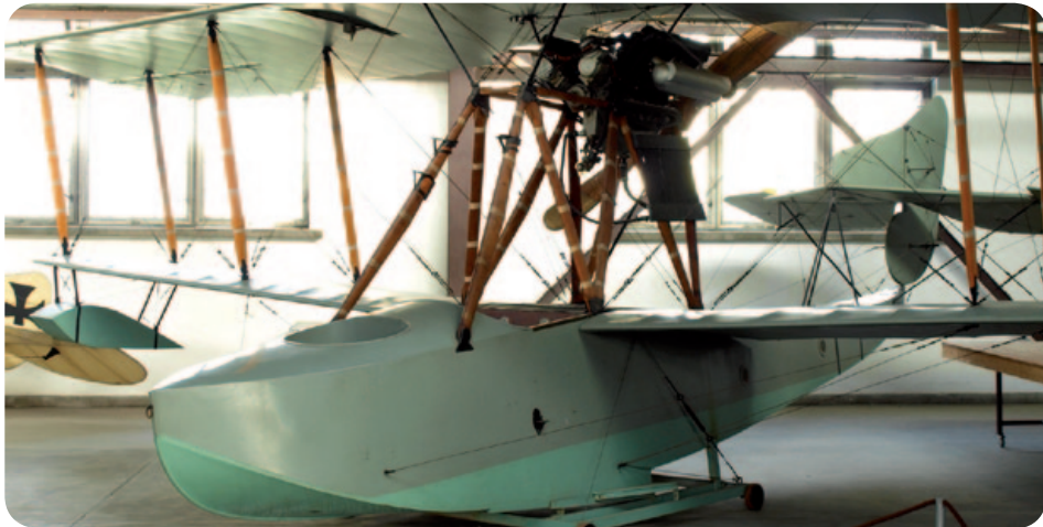
The Grigorovich M-15 a Russian two-seater reconnaissance flying boat was designed by Dimitri Grigorovich and produced in 1917 in St Petersburg for the Imperial Russian Navy. The aircraft on display is the only one of its kind preserved in the world. © Polish Aviation Museum in Krakow, photo by Jan Hofmann
